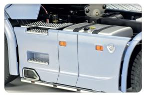
Side skirts also feature recreations of the indented steps. If desired, LEDs can also be installed in the marker lamps
