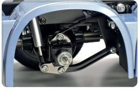
Axles are molded in reinforced plastic and supported by metal leaf springs, in a trunnion suspension like that seen on the real truck.
