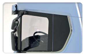
Just like on the full-size truck, the 2-sheet mirrors have 3D surfaces, recreated here with the use of metal-plated parts.
