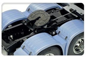
A coupler is installed on the back of the head to allow connection with one of the trailers in Tamiya's extensive line-up.
