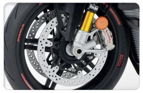
Take a closer look at the finely drilled brake rotors and brembo caliper.
