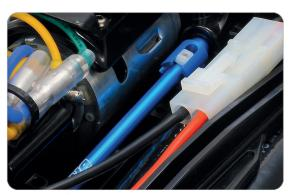
The kit features an aluminum propeller shaft with plastic inserts in the propeller joints to minimize wear.
