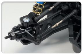
Assembly universal shafts help maintain speed when steering, for smoother cornering.
