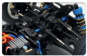
Turnbuckle steering and suspension arms can be adjusted quickly to fine-tune your setup.
