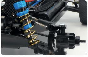
High spec oil dampers have precision aluminum cylinders with a low-friction interior coating.
